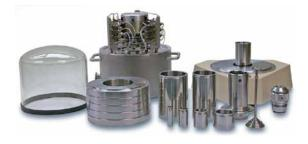
The AMH-38 provides automated mass handling of a 38 kg (84 lb)mass set for the PG7601 piston gauge platform. The mass handling system is integrated into a vacuum chamber which provides KF40 vacuum fittings for connection of a turbo molecular vacuum pump and external vacuum gauge if desired. Automated mass handling eliminates the need to break the vacuum between pressure points and reference vacuum as low as 0.01 Pa (< 0.1 mTorr) can be maintained indefinitely.
