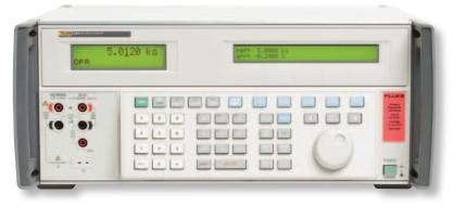
Using the 52120A Transconductance amplifier, the 5502E's output current is extended from 20.5 to 120 A; and with the use of 25 and 50 turn coils, it can calibrate instruments requiring currents up to 6000 A.
