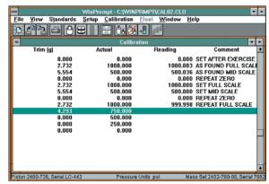
The WinPrompt calibration screen displays calibration values and allows for user comments. Export this information using dynamic data exchange (DDE) into your favorite word processing or spreadsheet program to create calibration certificates and reports.
