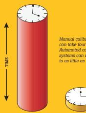
Manual calibration systems can take four hours or more. Automated calibration systems can reduce the time to as little as 15 minutes.
